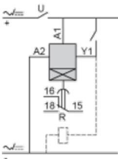
Function A : Power on Delay Relay
