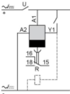
Function C : Off-Delay Relay with Control Signal
