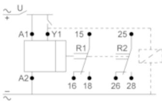
Function A : Power on Delay Relay
