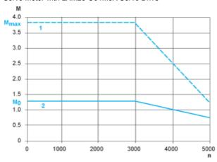
M: Torque in Nmn: Speed in rpm1: Peak torque2: Continuous torque
