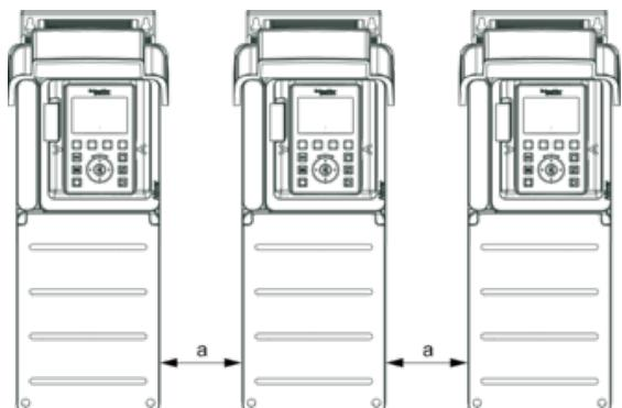
Mounting Type B: Side by Side IP20 , Only possible at ambient temperature lower than 40 °C (104 °F)
